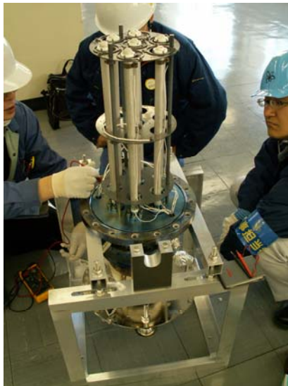
Internal structure of SO 3 electrolysis cell
